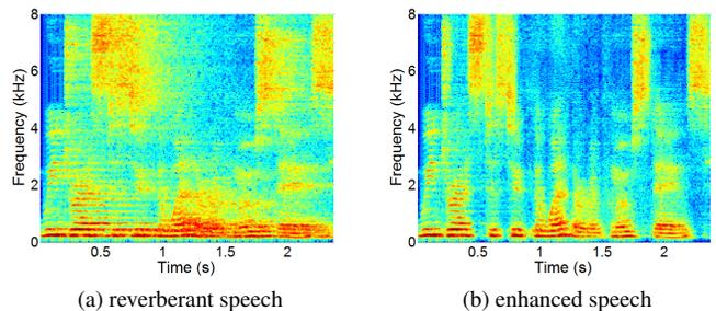
**Fig. 2:** (Color online) Example spectrograms of reverberant speech ( $T_{60} = 1.0$  s) and the corresponding enhanced speech.
