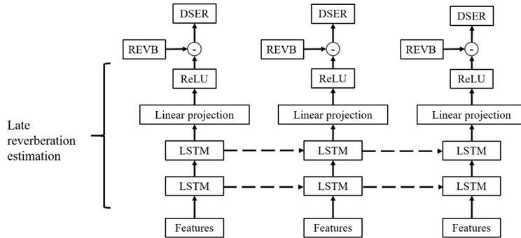
**Fig. 1:** System diagram of the proposed algorithm. “REVB” denotes the compressed magnitude spectrum of the reverberant speech; “DSER” denotes the compressed magnitude spectrum of the direct sound plus early reflections.
